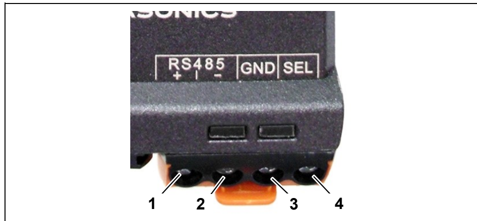
Fig. 7: Pin assignment, RS-485 and configuration connection Connector type: Weidmüller BHZ 5.00/04/90LH BK/OR
